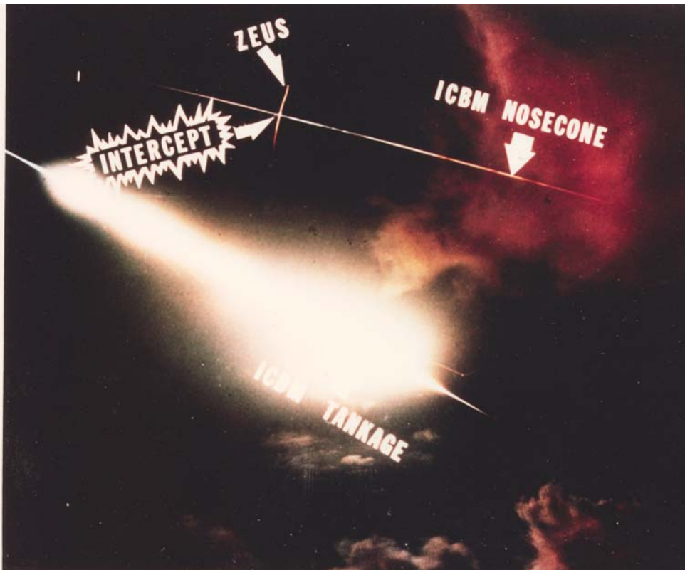
Fig. 2-9. An annotated photograph illustrating the Army's successful ICBM intercept.
