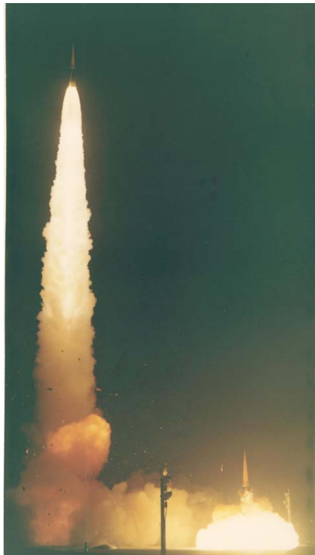
Fig. 2-31 and 2-32. During flight, the SPRINT missile achieved such speeds that it would become incandescent. SAFEGUARD tests included salvo tests for both missiles. A SPRINT salvo launch. (right)
